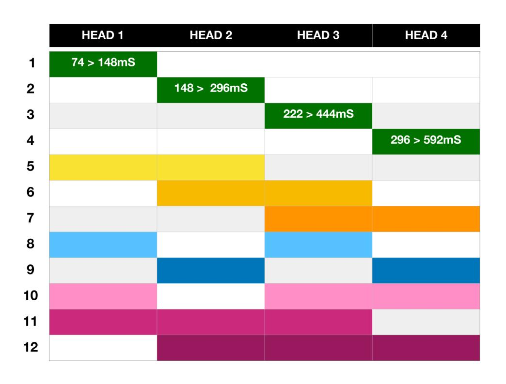
The minimum values shown in the table are with "varispeed" rotated in the 0% position, while the maximum values are 100%. The minimum values are with a 1% THD tolerance, while the maximum ones are 5%. However the synchronism of the heads remains very precise. The harmonic distortion ranges from 1% on the delay time 348mS to 5% in the maximum condition of 592mS.
