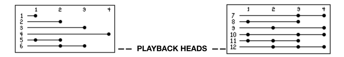
One example in Rep. mode: If you select the "5 position" switch, call together the fourth and third heads, it will mean the 4th Head considered as an 8th note, and 3rd head is equal to a dotted 8th. If you use the "varispeed" you can keep the synchronism by increasing the delay time over 100%.
