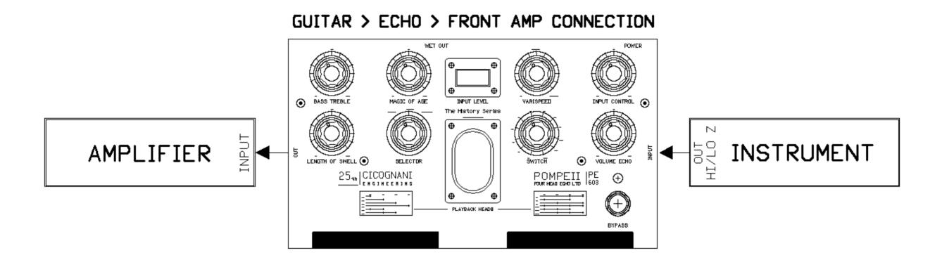
The use of the echo in front of the amplifier is one of the most classic configurations. Thanks to a powerful input and output buffer we can send a good and clean signal to the amplifier. The use of good quality cables is always recommended. If you use Fuzz, Od. or Dist. pedals move the echo to the end of the chain to obtain the best performance
