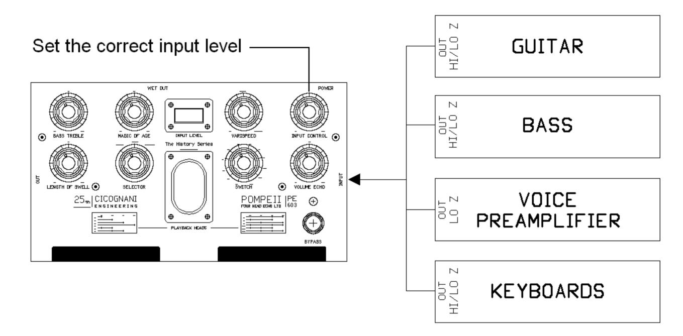
The Pompeii PE603 can be used with different types of instruments with output signals max 1Vpp and high or low impedances. The Old Italian echo was used as the main PA effect and shortly thereafter along with many instruments of the band. Today Pompeii wants to retrace those steps by offering wider compatibility even with the most modern instruments.
